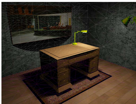
Figure 5: A typical problem caused by hemispherical projection. Although the shadow receiving surface (the wall) is tessellated highly enough, the shadow caster (the picture) is not. The bottom edge of the picture which is responsible for the shadow is a straight line in the projection and therefore leads to an elliptical shadow.
