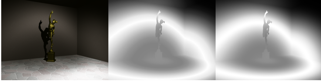
Figure 3.5.: Roman god mercury lit by a rotationally symmetric high-bay luminaire (left). The bilinear sampled light intensity from the LDT which is used for shading a surface point (middle) compared with the result of bicubic interpolation (right). White means maximum intensity whereas black is zero intensity. The goniometric diagram of the luminaire is depicted in Figure 3.6.
