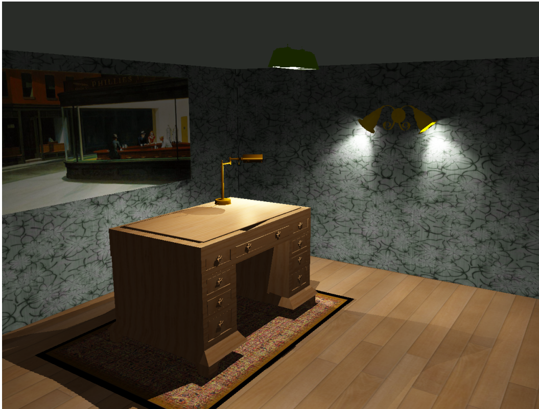
Figure 3.7.: A room lit by four goniometric light sources. Note the light distribution at the back wall, which does show a slightly anomalous spot light characteristic.
