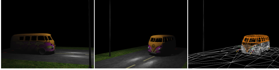
Figure 2.8.: The scene consists of 9012 triangles which are divided into 4259072 elements. The street lamp is simulated with a standard Lambertian light, the head and taillights are simulated with four spotlights. Each triangle was assigned a 32 \times 32 radiosity texture and shooting was done from the third mipmap level.
