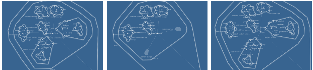
Figure A.7.: The initial layout of the graph is shown on the left. The clusters Western Europe and Eastern Europe are closed (middle). Their boundary are shrunk to 20% of their original size and their contents are hidden. If the clusters are reepend again the inflated clusters are arranged properly (right).
